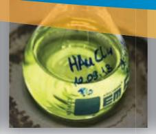
A solution containing gold from the pins of an old processor (Photo: iGEM Heidelberg 2013).
