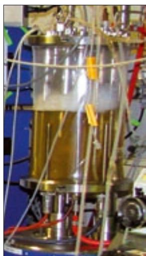
Cells are cultivated in the internal chamber and the medium in the external chamber can be renewed or exchanged as required.
