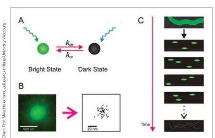
Photoswitchable fluorescent probes (A) can be switched between a fluorescent and a nonfluorescent state. Combining nanometer-precise localization of single molecules (B) and a temporal separation of the overall fluorescence signal (C) provides a large number of single-molecule coordinates which can be used to reconstruct a super-resolution image.
