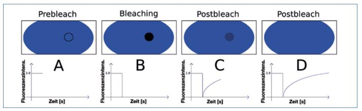
Diagram of a fluorescence recovery after photobleaching (FRAP) experiment. At the start of the experiment, a high-intensity laser beam is used to destroy irreversibly the fluorescence of the particles in a localised area. As time passes, the increasing fluorescence in that area provides information about the movement and reaction characteristics of the fluorescent particles being observed Image: UFZ
