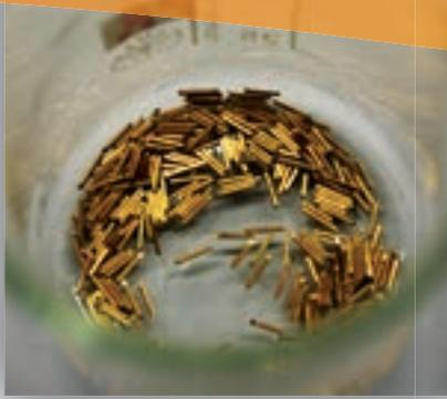
Contact pins from an old processor that contain gold (Photo: iGEM Heidelberg 2013).
